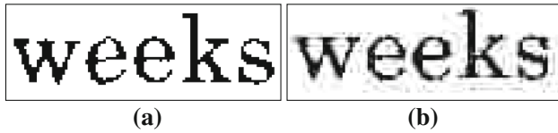
Fig. 2 Ringing artefact in JPEG coding algorithm ( q = 9 ): a original text; b reconstructed text
